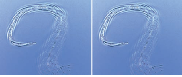
Fig. 2. Validation of our 3D iWave kernel: On the left is the result of a standard planar 2D iWave simulation after a figure-eight-shaped mouse input and 280 timesteps. On the right is the result of our 3D simulation after the same number of timesteps on the same input. Our simulation method introduces less than 1% error per timestep and produces visually indistinguishable results.
